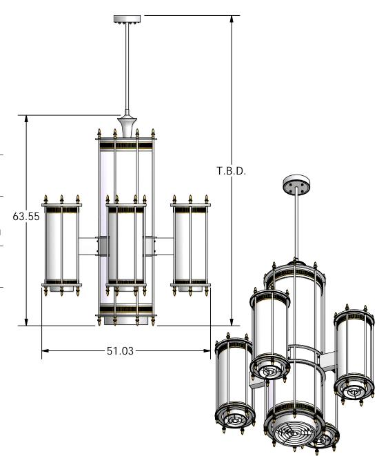
NOTES: ESTIMATED FIXTURE WEIGHT 250 LBS MOUNTS TO (4) 3/8-16 ANCHORS BY OTHERS. RIGID MOUNT. FIXTURE WIRED FOR 2 CIRCUITS
