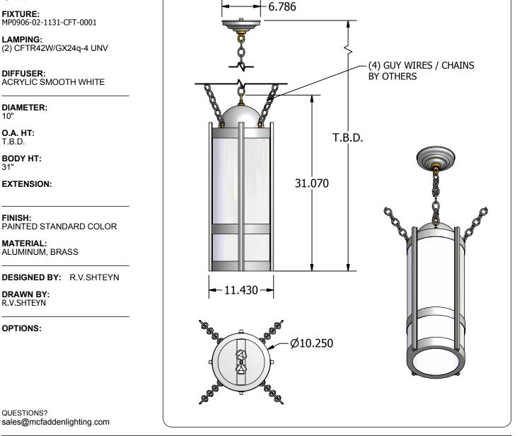
NOTES: FIXTURE EQUIPPED WITH (4) LOOPS FOR GUY WIRES/ CHAINS BY OTHERS
