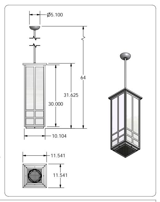
NOTES: PAR-38 250W QUARTZ HALOGEN LAMP OPEN FIXTURE RATED
