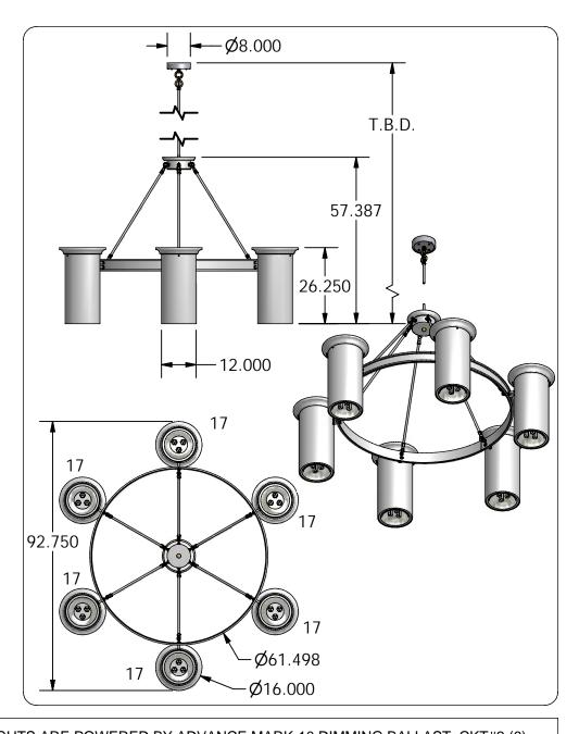
NOTES: CKT#1 (18) DOWN LIGHTS ARE POWERED BY ADVANCE MARK-10 DIMMING BALLAST. CKT#2 (6) UP LIGHTS NO DIMMING.
